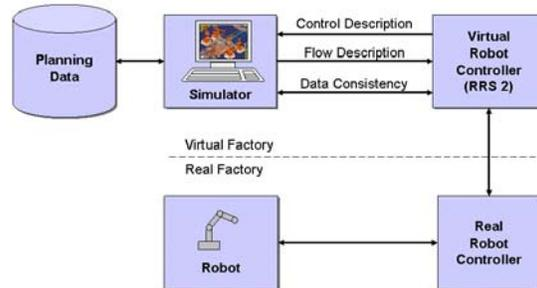
Figure 11: RRS (Realistic Robot Simulation) enables to use the real control algorithms in simulation.
