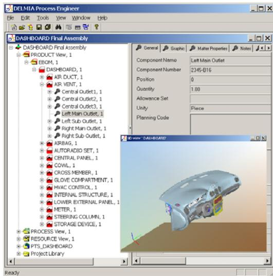
Figure 5: Product and process definition (Delmia)
