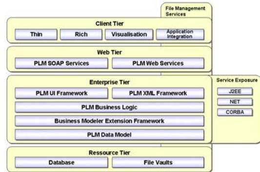
Figure 20: Factory data management architecture (UGS)
