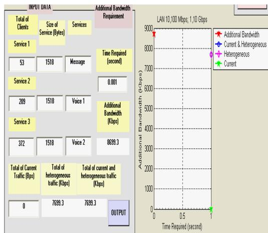
Figure 6.13: Network Traffic Management over Ethernet Technology Using Simulation Model Measurement (Time Series: 0.001 second) in Graphical Interface without Consider Any Current Traffic
