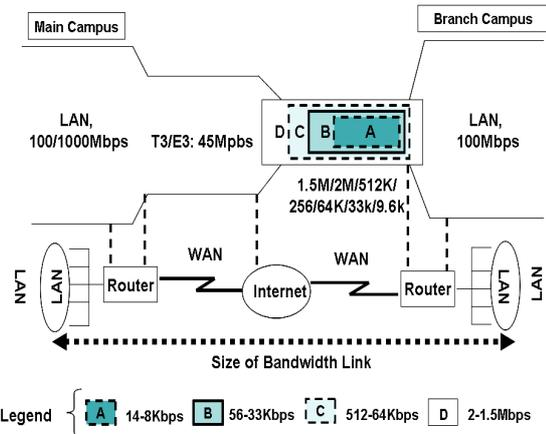
Figure 6.6: Bandwidth Link Capacity for LAN and WAN Measurement
