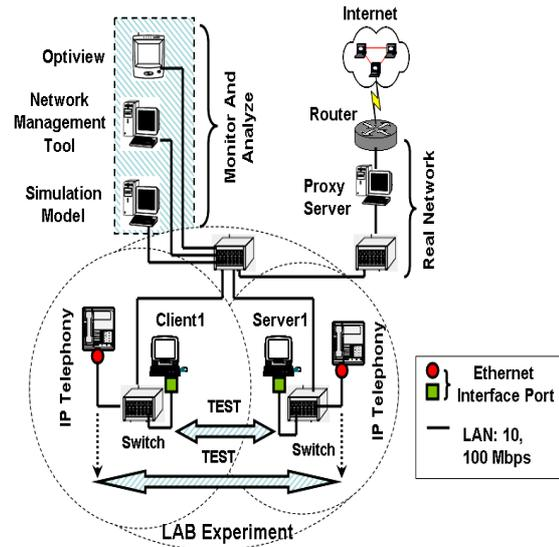
Figure 6.2: Experimental Laboratory for Network Environment Setup
