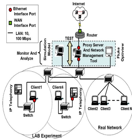
Figure 6.3: Experimental Laboratory for Real Network Environment Setup
