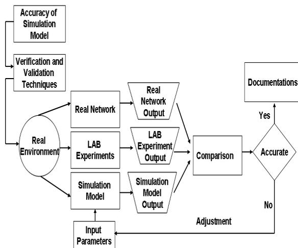
Figure 3.2: Simulation Model Verification and Validation Methodology
