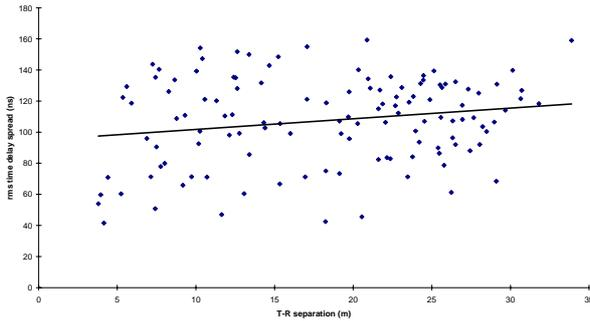
Figure 7. RMS time delay with distance
