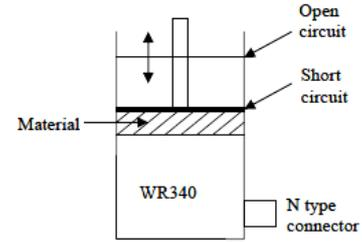
Figure 1. Waveguide sample holder
