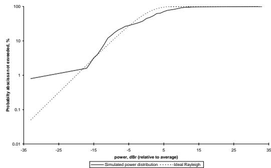
Figure 5. Simulated cumulative distribution function of power in the typical office
