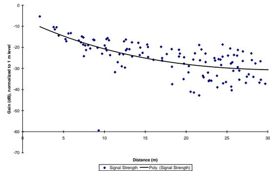
Figure 4. Signal Strength vs. distance in the typical office (1.8 GHz)
