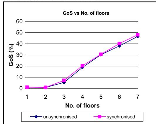
Figure 9. The performance of DCA (GoS) with up to seven service providers, one on each floor
