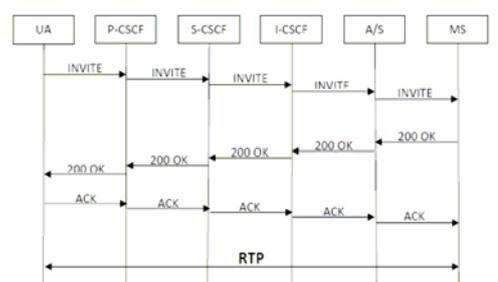
Figure 2: Simplified IMS Signalling
