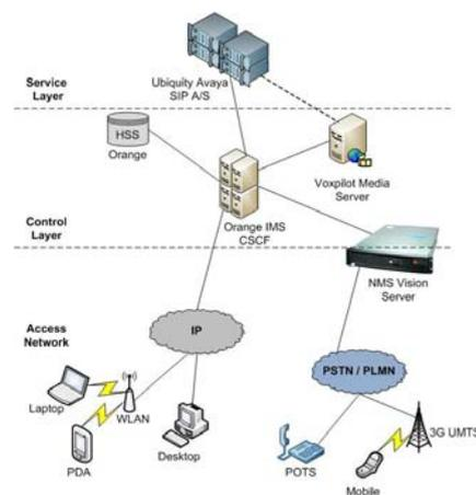
Figure 1: IMS Testbed Architecture
