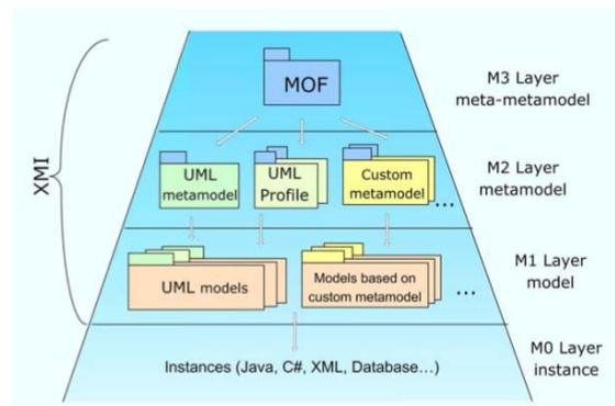
Figure 1. Structure of MDA (Miller and Mukerji, 2003).
