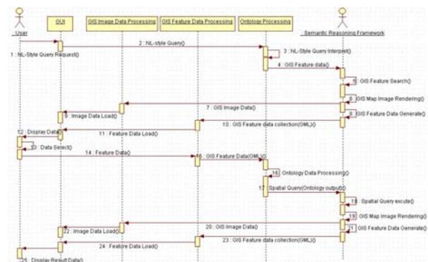
Figure 6. Sequence diagram for semantic query procedure.
