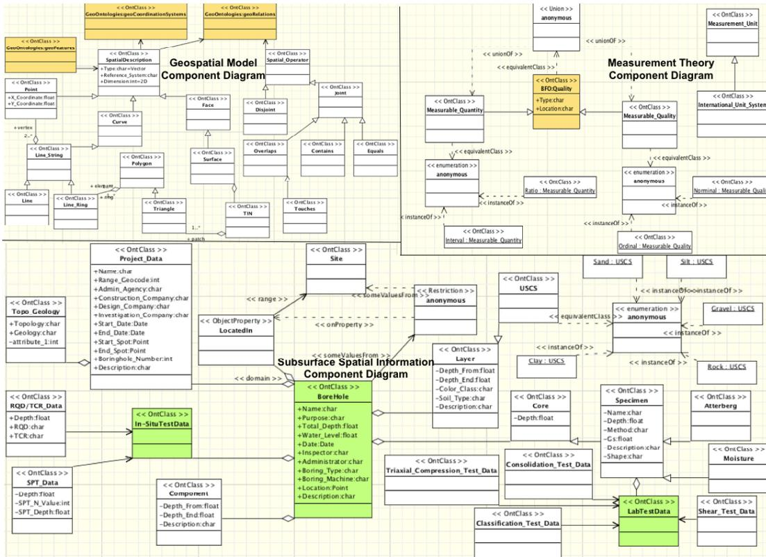
Figure 7. An excerpt of the UML profile model for subsurface spatial layer using Poseidon-UML.
