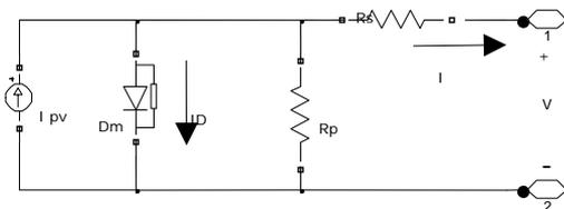
Figure 1. One-diode model.
