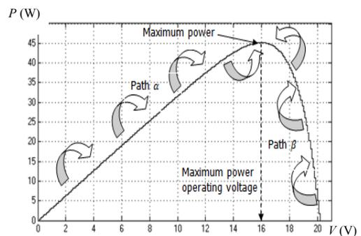
Figure 4. P&O tracking path.
