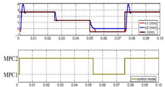
Fig. 8. Switching MPC control system: (1) position of masses and (2) switching signal [3].
