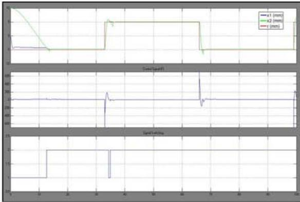
Fig. 5. Switching PID control system: (1) position of masses, (2) control signal (F) and (3) switching signal.
