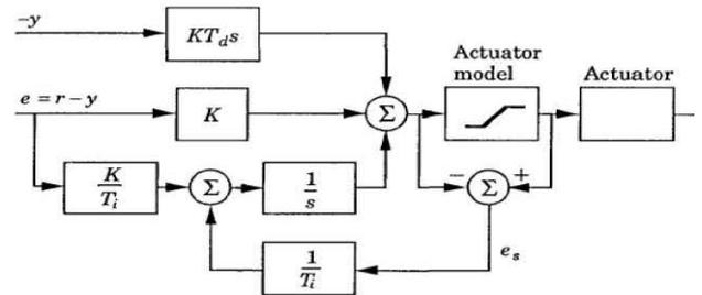
Fig. 3. PID Controller with anti-windup [7].
