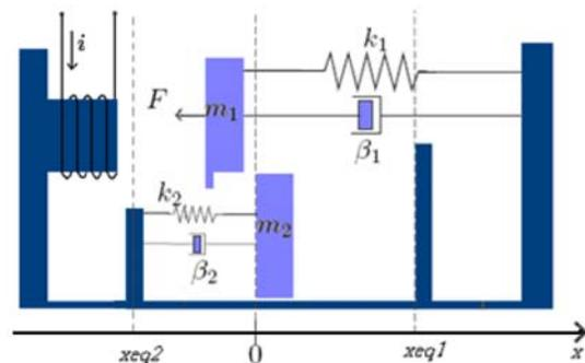
Fig. 1. Mass spring damper system schematics [3].
