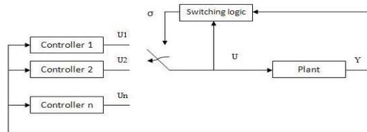
Fig. 4. Block Diagram of a Switching System
