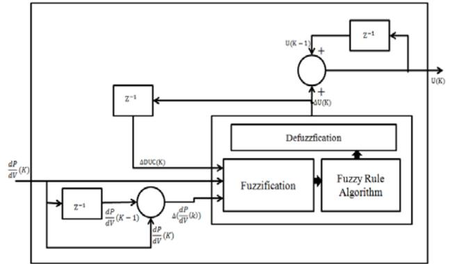
Figure 6: Functional block diagram of fuzzy logic controller (FLC)
