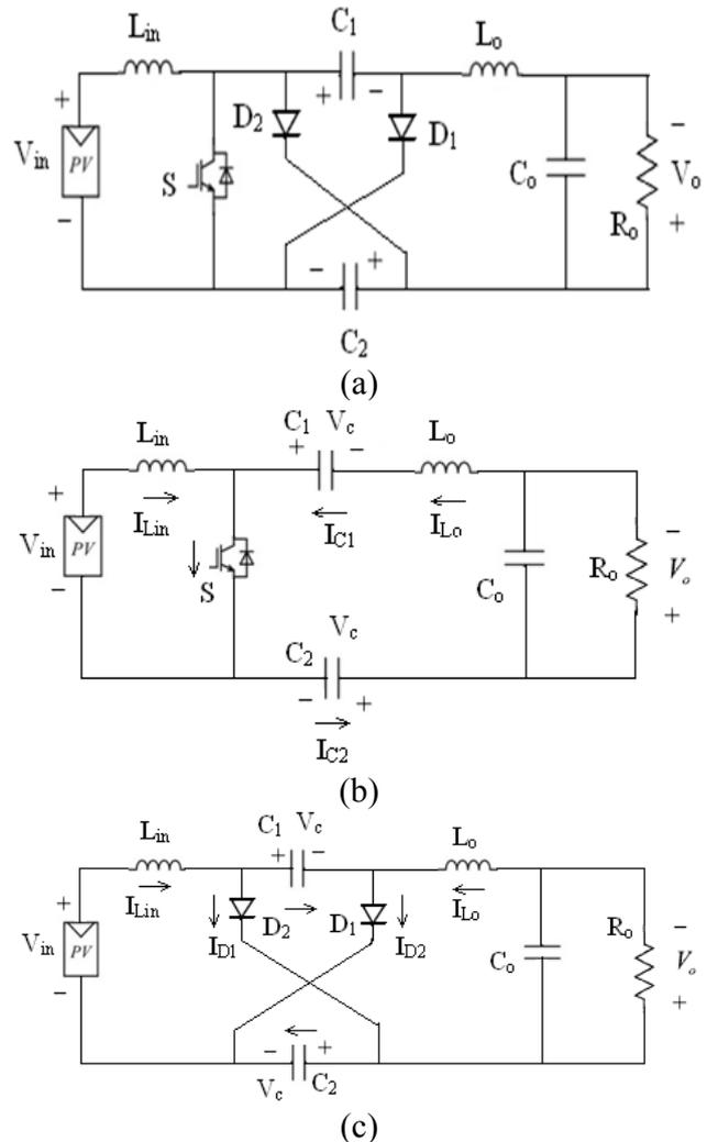
Figure 5 (a) Converter diagram (b), (c) Converter switching topologies (t<sub>on</sub> & t<sub>off</sub> mode)
