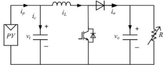
Figure 3: Circuit of a boost converter
