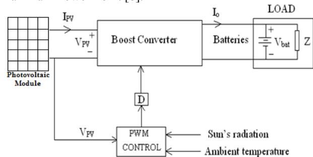
Figure 1: Typical MPPT Controller
