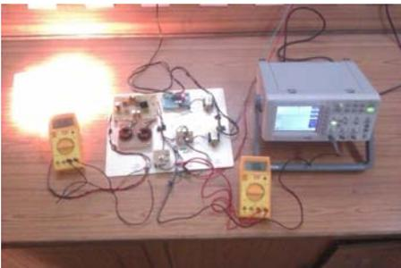
Figure 11: Experimental setup showing controller integrated with the Solar PV Panel
