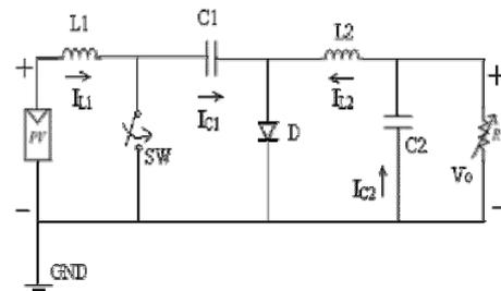
Figure 4: Circuit diagram of conventional cuk converter
