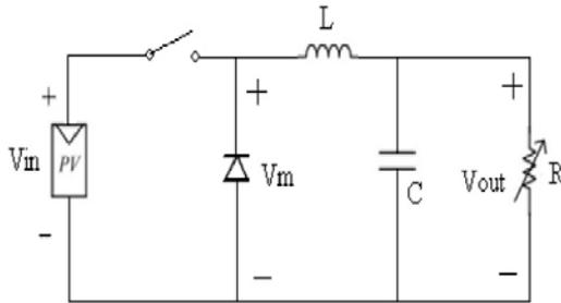
Figure 2: PV Array with buck converter circuit diagram
