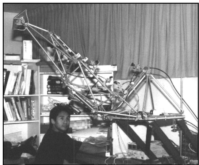
Figure 2. VGTM robot leg fully extended
