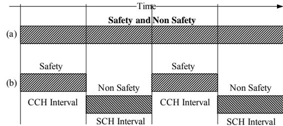
Figure 2. Single-channel and multi-channel operation
