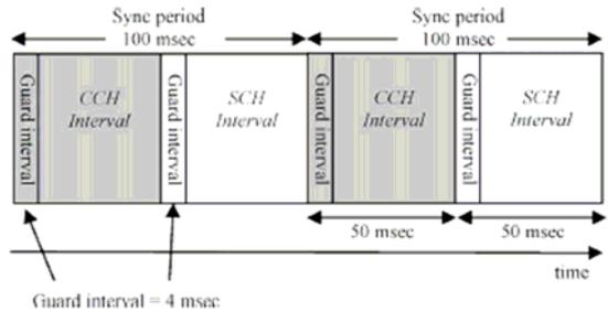
Figure 1. Allocation CCH interval and SCH interval [12]
