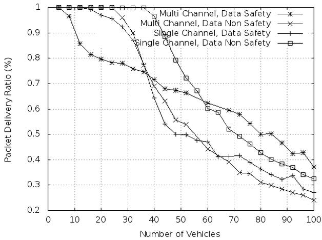
Figure 9. The comparison between the packet delivery ratio single-channel and multi-channel
