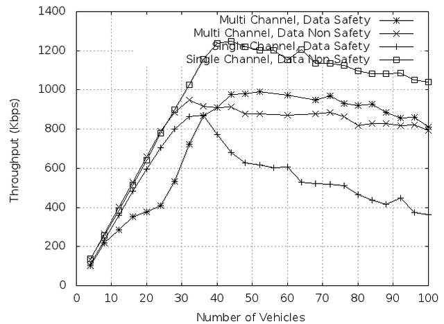
Figure 11. Comparison of throughput single-channel versus multi-channel
