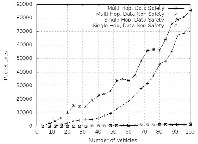
Figure 14. Comparison of packet loss single-hop versus multi-hop
