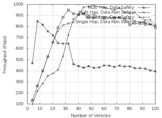
Figure 15. Comparison of throughput single-hop versus multi-hop
