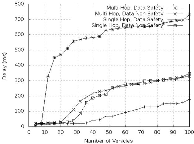
Figure 12. Comparison of delay single-hop versus multi-hop
