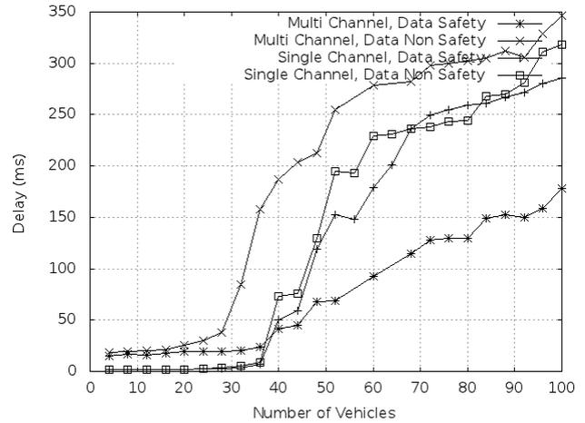
Figure 8. Comparison of delay single-channel versus multi-channel
