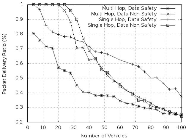
Figure 13. Comparison of packet delivery ratio single-hop versus multi-hop
