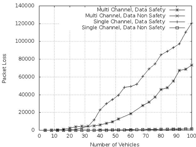
Figure 10. Comparison of packet loss single-channel versus multi-channel
