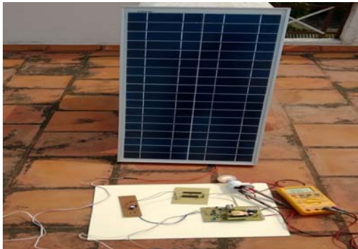
Figure 29. Interleaved converter with MPPT control
