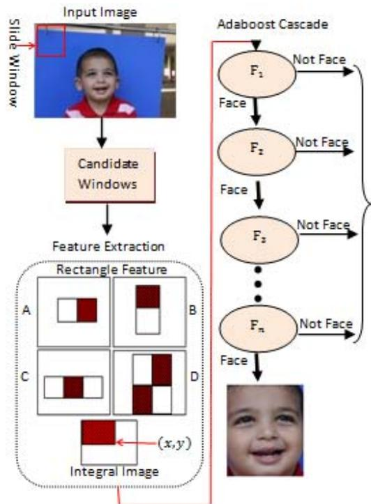
Fig. 1 : Face Detection Algorithm: Four Rectangular Features (a, b, c, and d).
