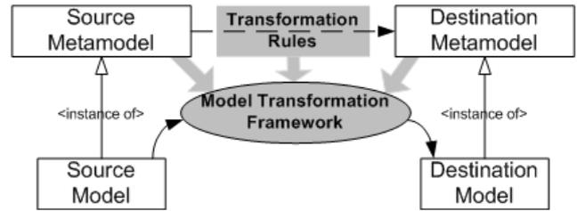
Fig. 3 : Model Driven Architecture.
