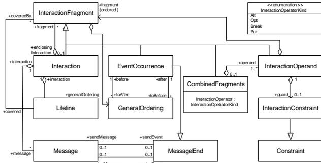
Fig. 1 : Sequence Diagram Metamodel.
