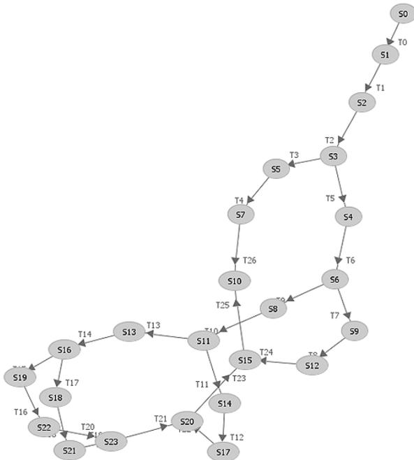
Fig. 8 : Reachability Graph Generated using PIPE.
