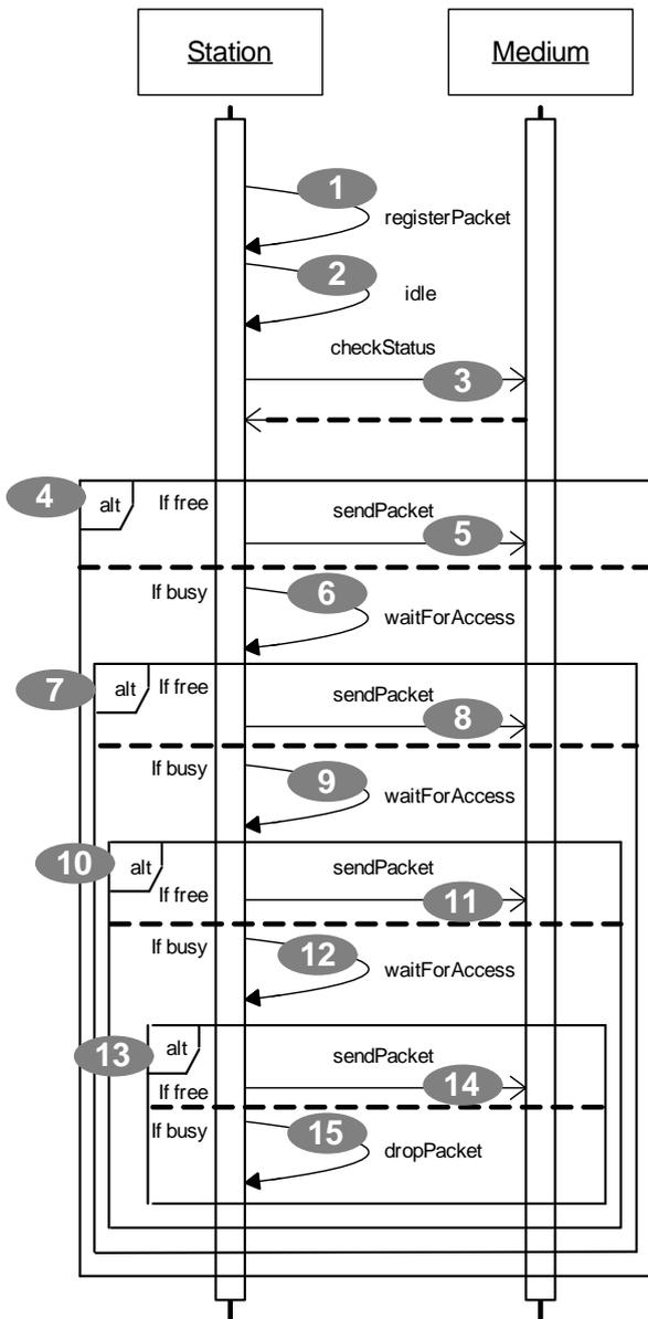
Fig. 6 : Sequence Diagram of the IEEE 802.11 CSMA/CA Protocol.
