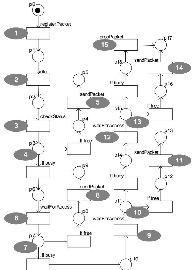
Fig. 7 : Petri Net of the IEEE 802.11 CSMA/CA Protocol Generated by SD2PN.
