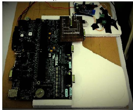
Figure 3. Prototype of the controller circuits
