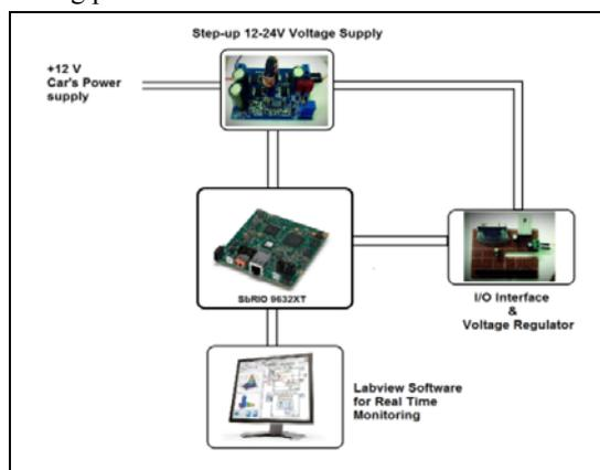
Figure 2. Block diagram of the monitoring system
