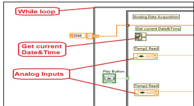
Figure 8. Analog data acquisition
