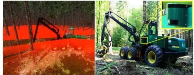
Figure 21. Screenshot of the virtual harvester testbed equipped with 2D LiDAR scanners for forest navigation and harvesting support (left) and the real world setup that was realized after detailed testing and optimization in the virtual testbed (right).
