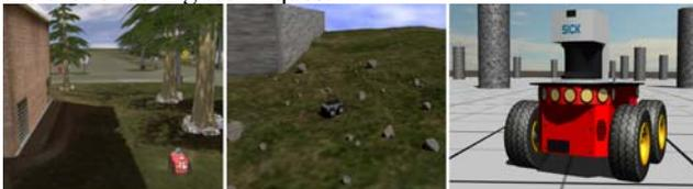
Figure 2. Screenshots of current robot simulators. Left: USARSim, middle: Gazebo, right: Webots. Images taken from the developers' websites.
