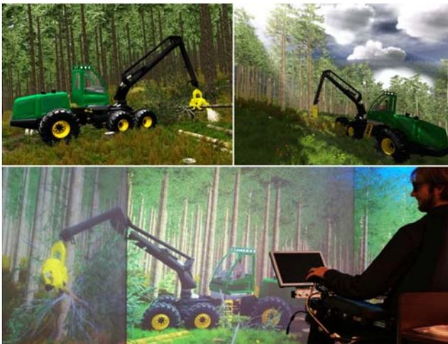
Figure 18. Current wood harvester simulator, which applies a virtual mapping of the real world environment to increase training effectiveness.
