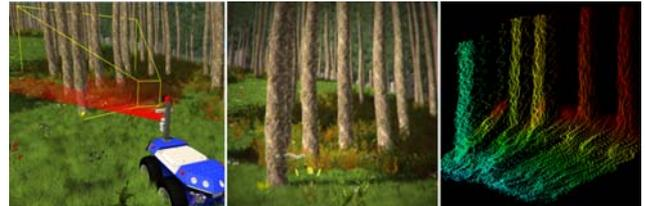
Figure 19. Simulation of the SeekurJr mobile robot platform and results of the simulated stereo camera (middle) and a ToF camera (right).
