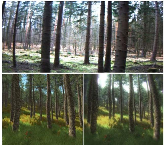
Figure 12. Comparison of an image taken with the Bumblebee XB3 stereo camera (top) and the corresponding rendered image without (bottom left) and with (bottom right) the simulation of typical camera effects.
