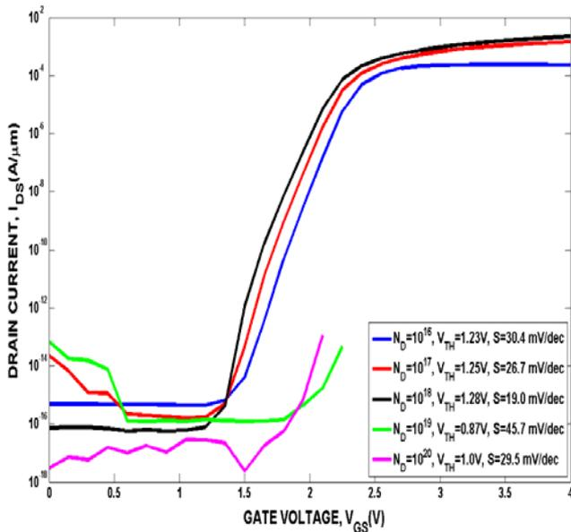
Figure 4. Transfer Characteristics,  $I_{DS}$ - $V_{GS}$  of VESIMOS-DP for  $Si_{0.7}Ge_{0.3}$ , S/D doping =  $2.0 \times 10^{18}/cm^3$ ,  $N_A = 4.0 \times 10^{19}/cm^3$   $V_{DS}=1.75V$  at different S/D doping concentration.
