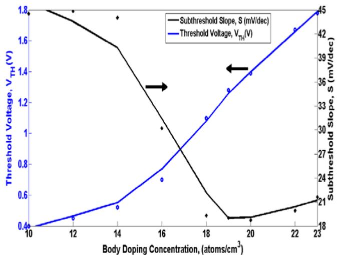
Figure 7. VESIMOS-DP Threshold Voltage and Subthreshold slope variation at different body doping concentration..
