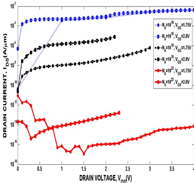
Figure 8. Output characteristics of VESIMOS-DP for  $\text{Si}_{0.7}\text{Ge}_{0.3}$ , S/D doping  $=2.0 \times 10^{18}/\text{cm}^3$ ,  $V_{GS}=1.75\text{V}$  and  $V_{GS}=2.0\text{V}$  at different body doping concentration.
