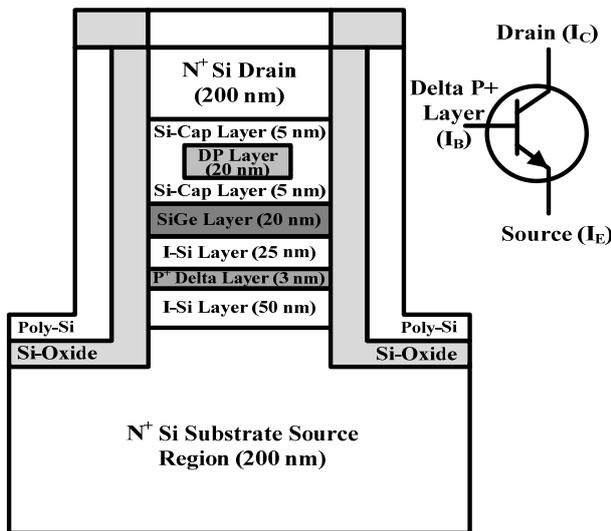
Figure 1. VESIMOS-DP device structure with respective layer thickness of source, drain, δp<sup>+</sup>, i-Si, SiGe, Si-cap and DP.
