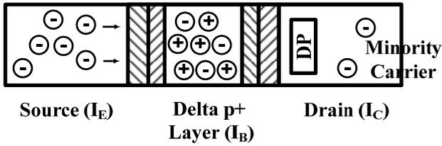
Figure 2. Parasitic Bipolar Transistor (PBT) effect principle of VESIMOS-DP device in Bipolar (BJT) mode.
