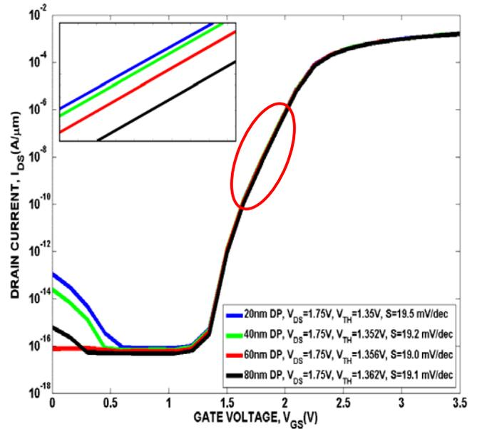
Figure 3. Transfer Characteristics,  $I_{DS}-V_{GS}$  of VESIMOS-DP for  $Si_{0.7}Ge_{0.3}$ ,  $S/D$  doping =  $2.0 \times 10^{18}/cm^3$ ,  $N_A = 4.0 \times 10^{19}/cm^3$ ,  $V_{DS}=1.75V$ .
