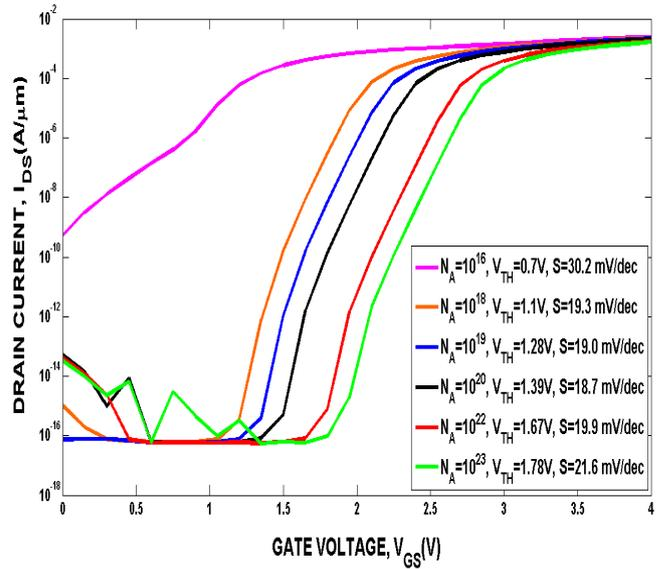
Figure 6. Transfer Characteristics,  $I_{DS}$ - $V_{GS}$  of VESIMOS-DP for  $\text{Si}_{0.7}\text{Ge}_{0.3}$ , S/D doping =  $2.0 \times 10^{18}/\text{cm}^3$ ,  $N_A = 4.0 \times 10^{19}/\text{cm}^3$ ,  $V_{DS} = 1.75\text{V}$  at different body doping concentration..
