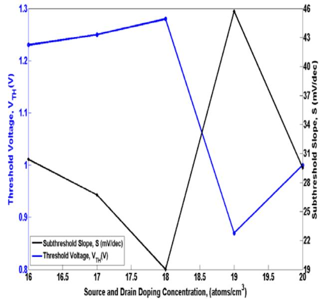
Figure 5. VESIMOS-DP Threshold Voltage and Subthreshold slope variation at different S/D doping concentration.
