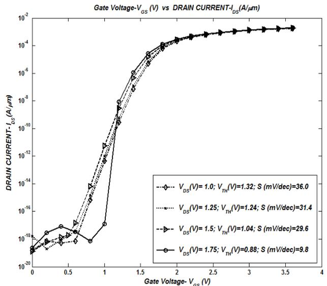
Figure 4. Transfer Characteristics of VESIMOS for  $\text{Si}_{0.7}\text{Ge}_{0.3}$ , S/D doping =  $2.0 \times 10^{18}/\text{cm}^3$ .
