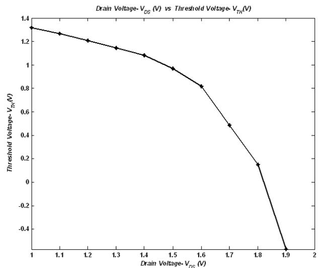
Figure 6. VESIMOS Drain voltage ( $V_{DS}$ ) vs. Threshold.
