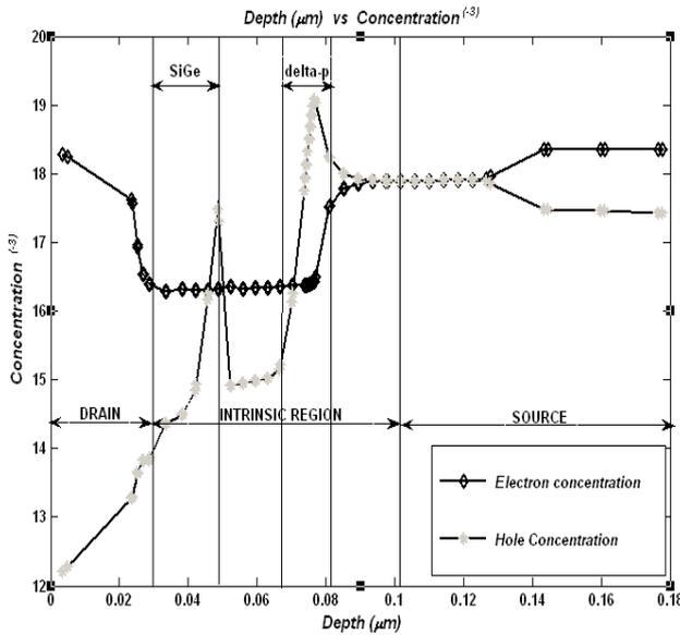
Figure 7. Electron and hole concentrations in different regions of the device.
