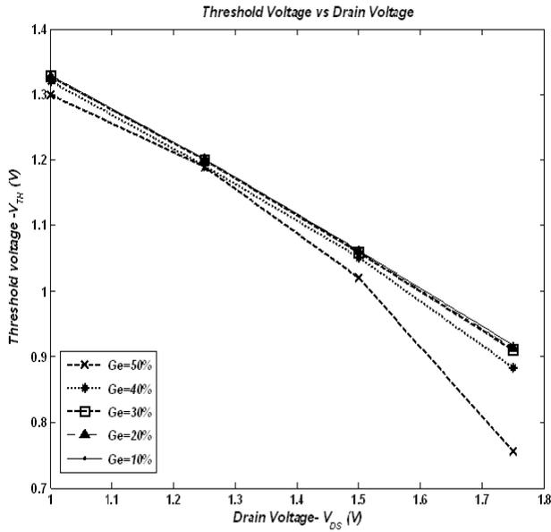
Figure 9. Variation of threshold voltage with Ge content.
