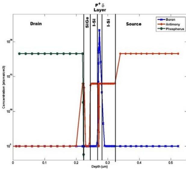
Figure 2. SIMS profile showing the doping concentration in different regions of the VESIMOS-DP structure.
