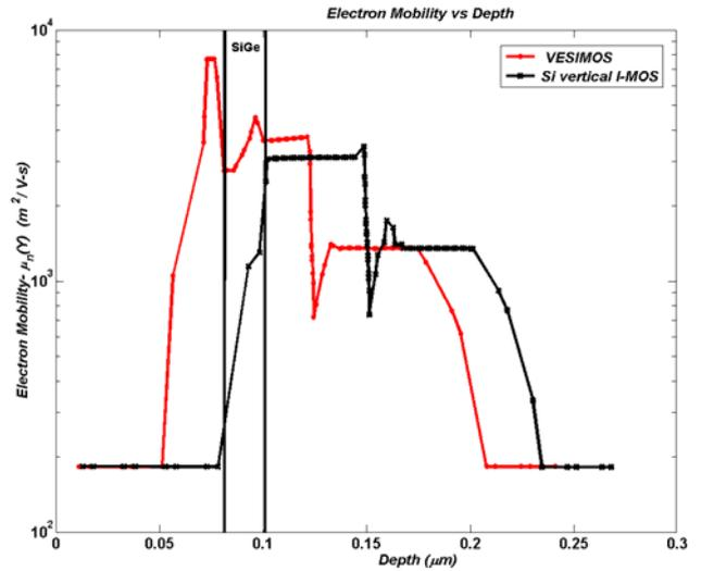
Figure 8. Comparison of electron mobility profiles of VESIMOS and relaxed Si vertical I-MOS.
