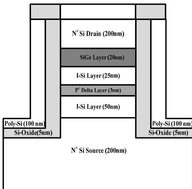
Figure 1. VESIMOS device structure with dimensions,  $d=0.8\mu\text{m}$ ,  $L=0.5\mu\text{m}$ , respective layer thickness of source, drain,  $\delta p^+$ , i-Si, SiGe and Ge=30%.
