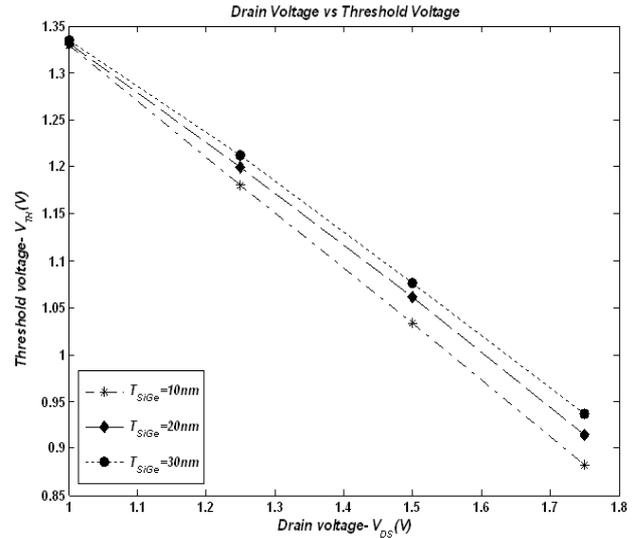
Figure 10. Variation of threshold voltage with Si<sub>0.7</sub>Ge<sub>0.3</sub> layer thickness.
