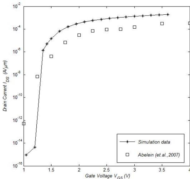
Figure 12. Validation of simulated data with experimental data (Abelein *et al.*, 2007) of Si vertical I-MOS device.
