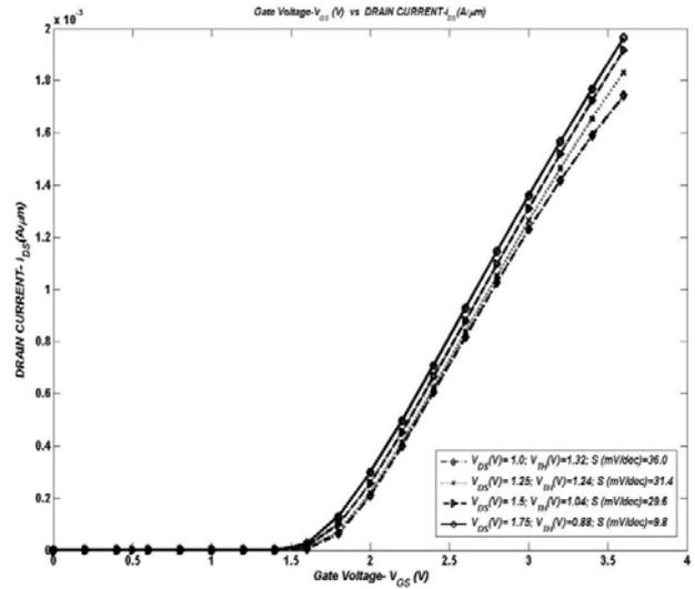
Figure 3. Current-Voltage characteristic of VESIMOS for  $\text{Si}_{0.7}\text{Ge}_{0.3}$ , S/D doping =  $2.0 \times 10^{18}/\text{cm}^3$ .
