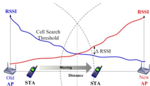
Figure 2. Initiation of handoff process when STA move away from current attached AP (old AP) [5]
