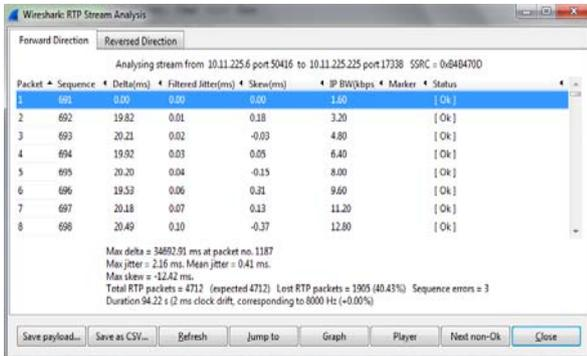
Figure 12. RTP Streaming analysis
