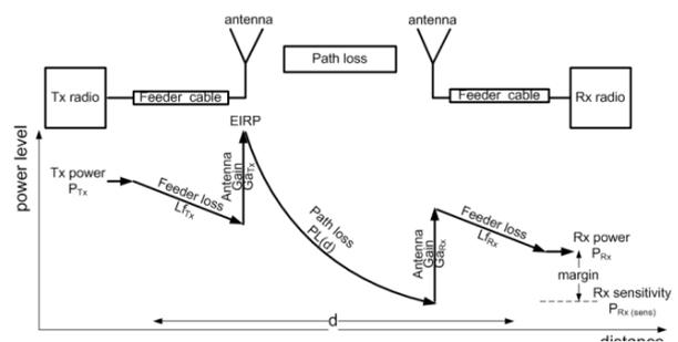
Figure 1. Power link budget in radio system
