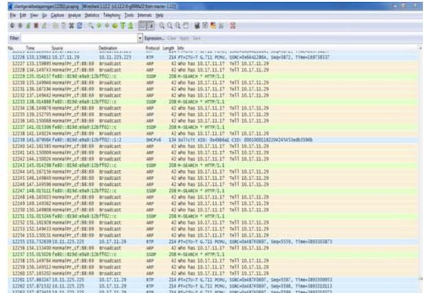
Figure 10. Screenshot of Wireshark during inter-subnet handover phase
