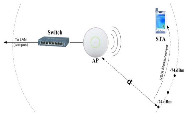
Figure 4. Measurement of  $P_{Rx\ sensitive}$  to get coverage area of AP
