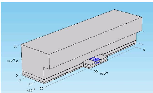
Fig. 7-One quarter of the SPC in WR90 waveguide, ready to simulate.
