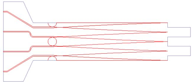
Fig. 4 – A card with four antipodal FLuS's and a p-QWT.
