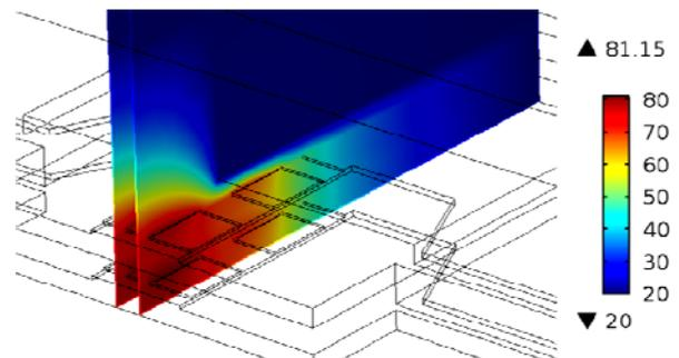
Fig.10-Temperature [°C], with Copper carriers and uniform power distribution: zoom view.
