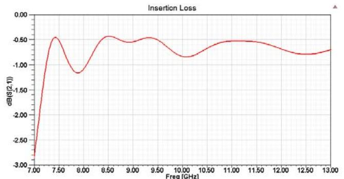
Fig.15-The simulated insertion loss of the passive SPC.
