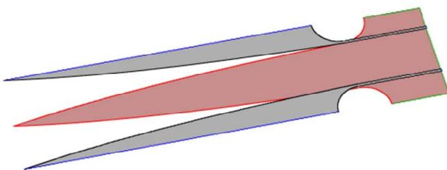
Fig. 3 – Double FLuS in antipodal configuration.
