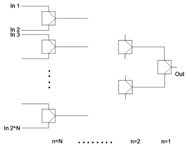
Fig. 2– The binary approach for a Power Combiner.
