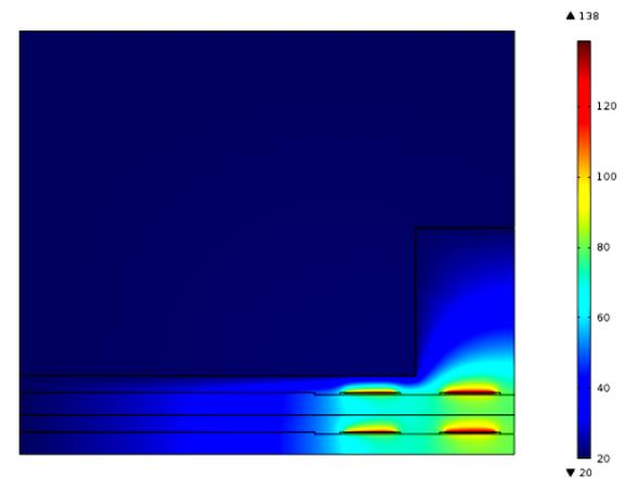
Fig.9-Temperature [°C], with Copper carriers.
