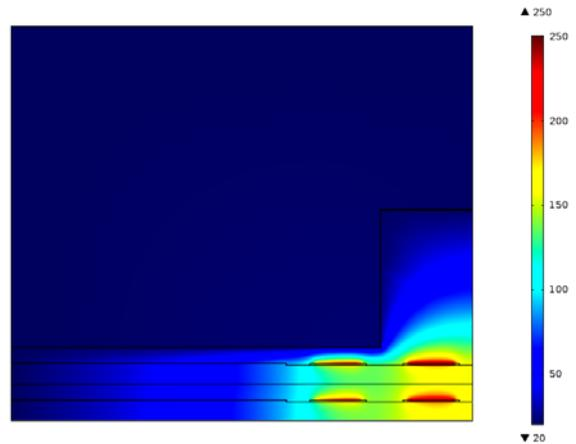
Fig.8-Temperature [°C], with Aluminum carriers.
