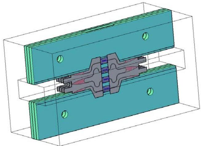
Fig.6-Three carries, 16 MMIC's, inserted in a WR90 waveguide.
