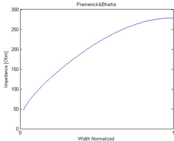
Fig.5-Taper impedance vs. taper width computed by the custom software.
