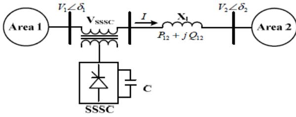
Fig.2 Schematic of interconnected two-area power system with SSSC in series with tie-line.
