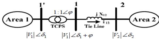
Fig.5 Schematic of interconnected two-area power system with TCPS in series with tie-line
