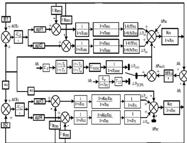
Fig.1 Block diagram of two area multi unit hydro thermal power systems.
