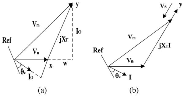
Fig.3 Phasor diagram (a)  $V_s = 0$  (b)  $V_s$  lagging  $I$  by  $90^\circ$ .
