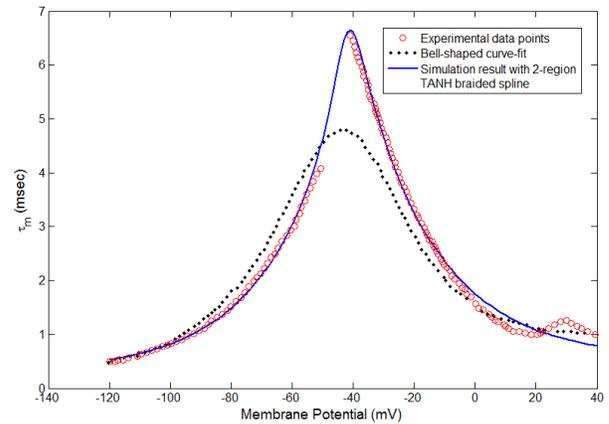
Figure 2. Proof of concept of implementation of two-region TANH interpolation technique, indicated in blue solid line. The red circles represent the experimental activation time constants for TTX-R persistent channels in spinal sensory neurons; the black dotted line depicts the bell-shaped curve that the authors had chosen to fit their experimental data. The latter two have been manually digitized from Figure 2E in Herzog *et al.* [12].
