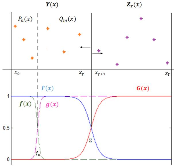
Figure 3. Graphical representation of the three-region TANH spline interpolation technique.
