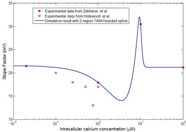
Figure 5. The curve fit obtained for the slope factor data (red filled circles) taken from Figure 6A of Zakharov *et al.* [18] after interpolating with two-region TANH spline (blue solid line). The graph also plots the additional experimental slope factor data that was procured from Hollywood *et al.* [19] (red unfilled circles).
