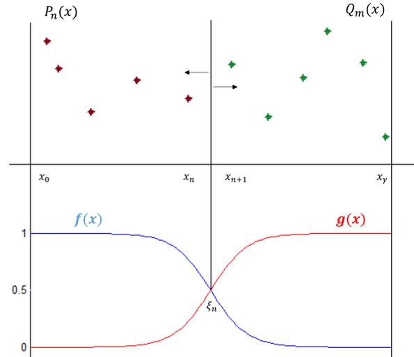
Figure 1. Graphical representation of the two-region TANH spline interpolation technique.
