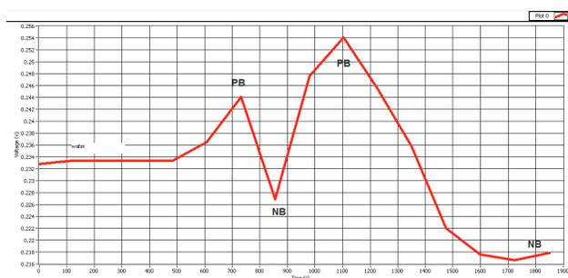
Figure 7: The fluorescence signal for the positive and negative bacteria, with high concentration and DI water after encapsulation.
