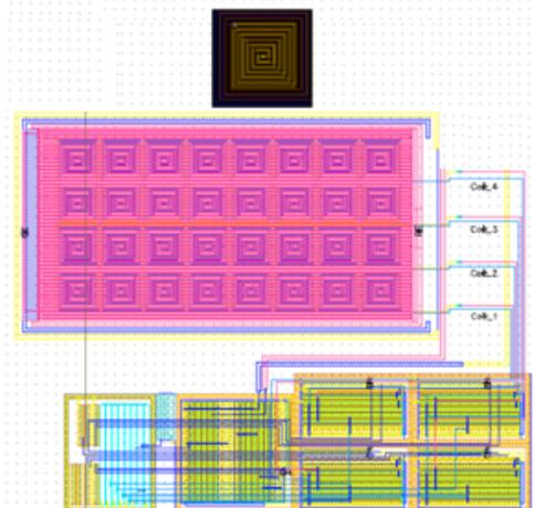
Figure 5: Layout of the magnetic generator along with the control signal and current source circuits.
