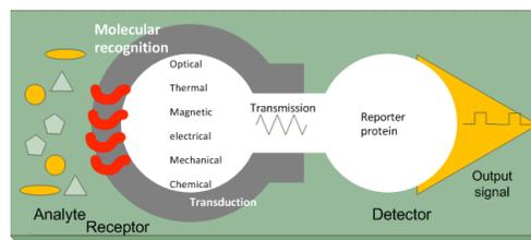
Figure 1: General model for biosensors, differentiating between molecular recognition, transduction and data processing.
