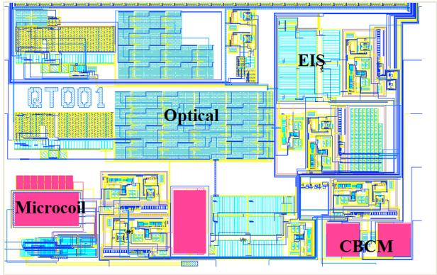
Figure 2: Layout of the entire multibiosensor device on a single chip.
