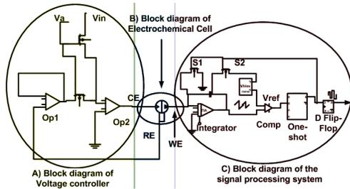
Figure 3: Circuit diagram of EIS.
