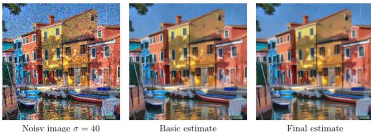
Fig. 12. Example of the BM-3D algorithm at work. From left to right: noisy source image, image after step 1 and image after step 2[19].
