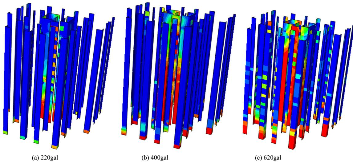
Figure 2. Final tension damage chart of wall under different seismic peak.
