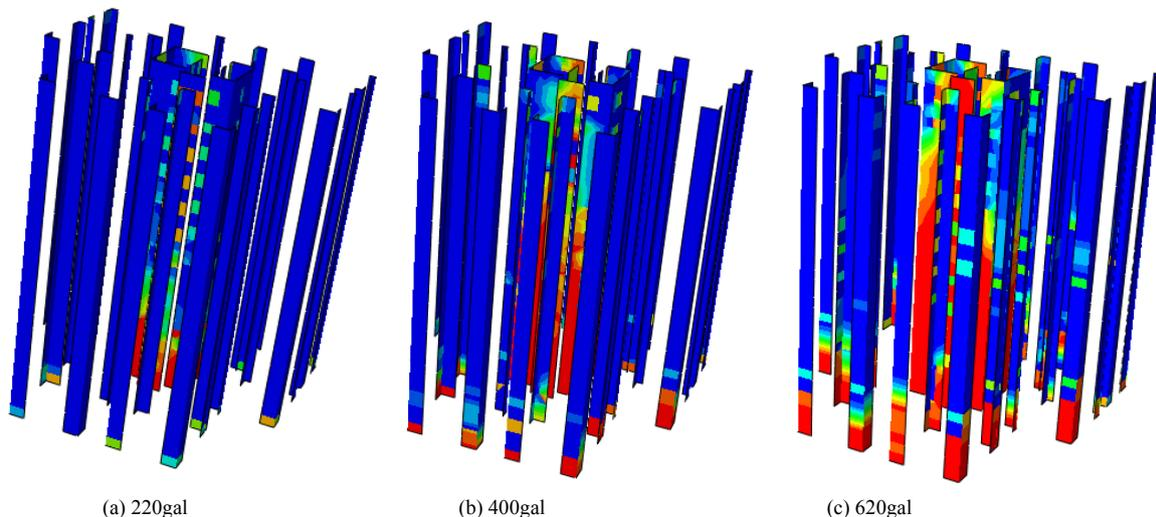
Figure 5. Tension damage chart of A3 wavelet
