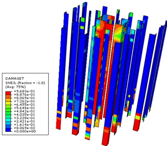
Figure 3. First order resonance failure state diagram of structure.
