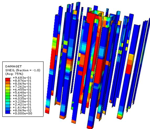
Figure 4. Fourth order resonance failure state diagram of structure.
