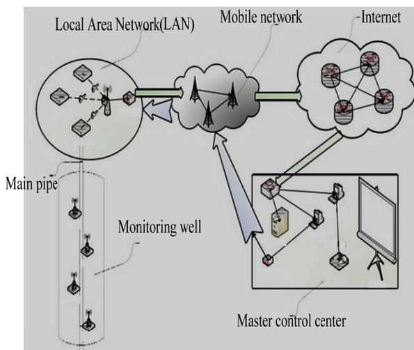
Figure 2. Shallow ground temperature monitoring network
