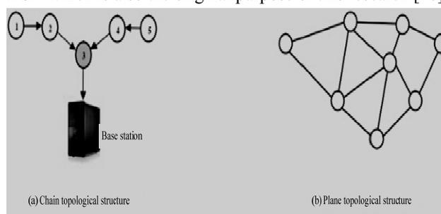
Figure 4. Chain topological structure and plane topological structure
