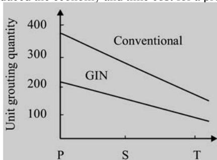
Figure 2. The unit grouting quantity of conventional and grouting intensity number methods.
