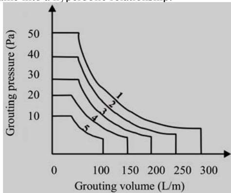
Figure 1. Grouting restricted envelope line.
