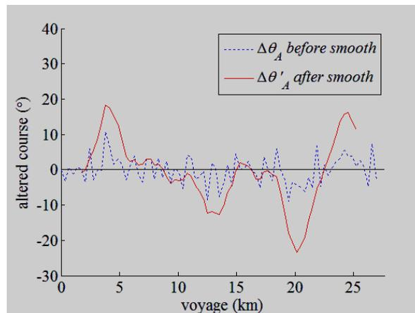
Figure 2. Curve smoothing of course alteration of trajectory  $A$ .
