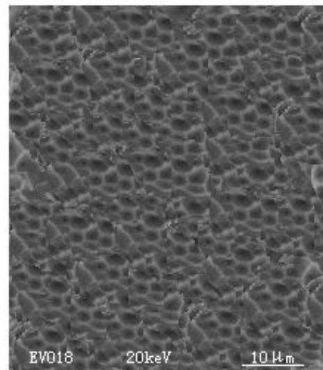
Figure6. 350°C temperature tensile fracture of specimens SEM picture
