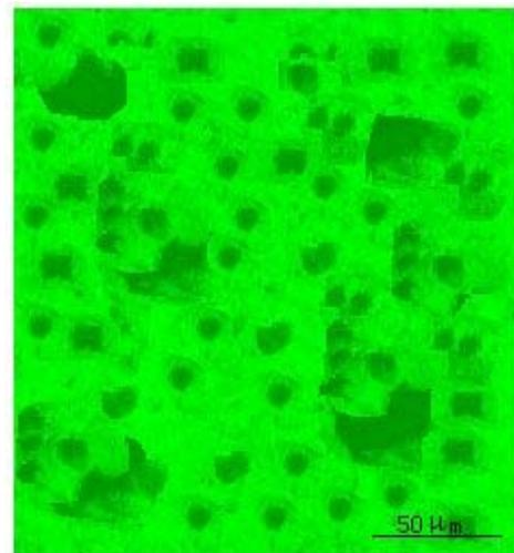
Fig. 8 Surface morphology after the AZ31 magnesium alloy corrosion
