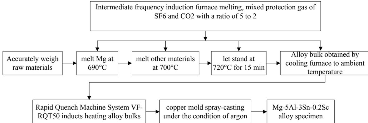
Figure1. Schematic of Melting Unit
