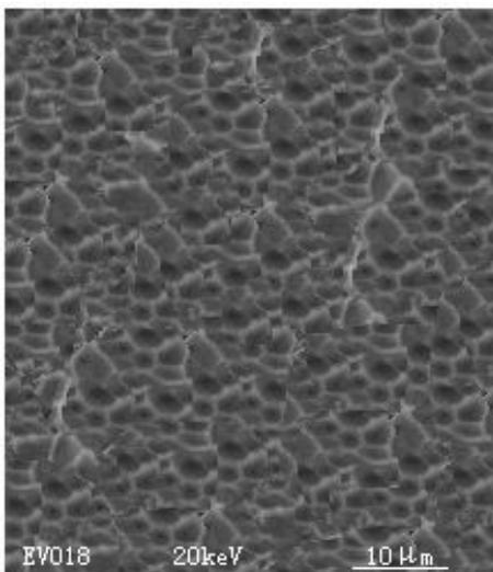
Figure5. Room temperature tensile fracture of specimens SEM picture
