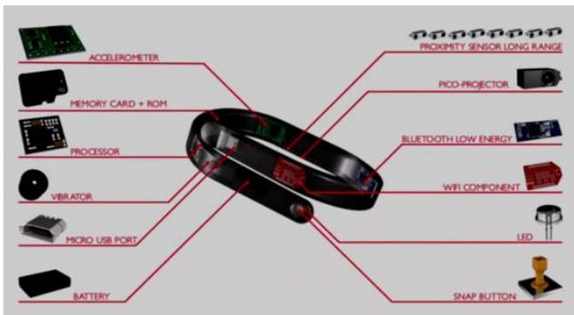
Figure 1. The structure of a smart bracelet called DS190.
