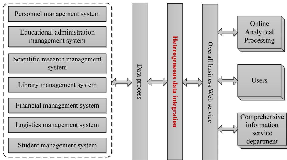
Figure 3. Architecture of the digital campus information sharing platform
