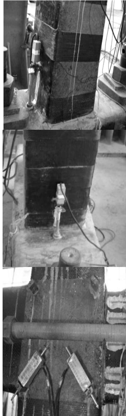
Figure 4 The displacement meter (the rotation of column base)
