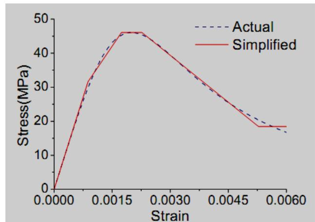
Figure 6. The simplified constitutive model of concrete
