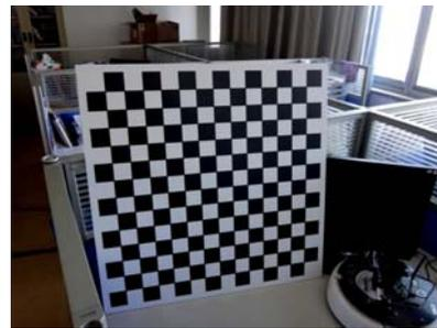
Figure. 7 The plane pattern of camera calibration
