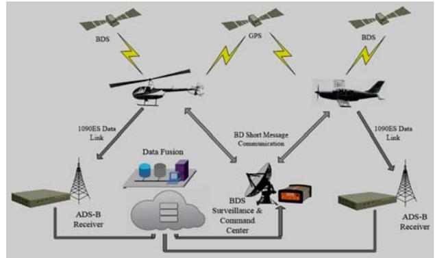
Figure1. The principle diagram of system
