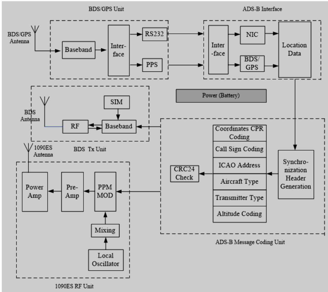
Figure 2. The principle of airborne device
