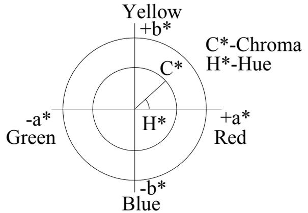
Figure.6 The simplified model illustration of  $L^* a^* b^*$
