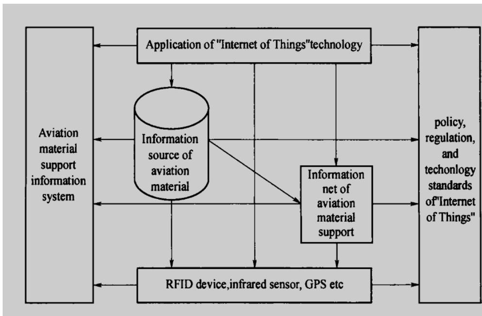
Figure 1. Aviation material supply information platform based on "Internet of Things".
