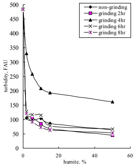
Figure 7. Effect of humite/0.5%APAM double grouping on turbidity
