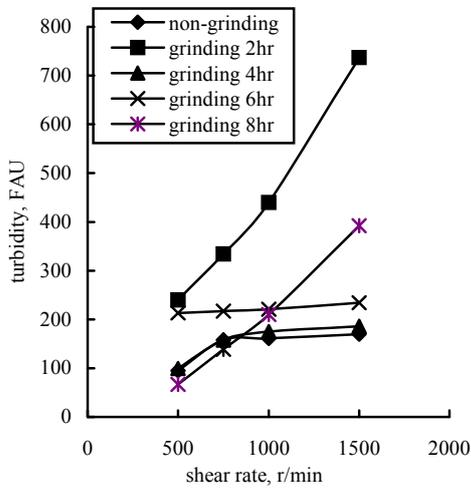
Figure 8. Effect of shear rate on turbidity of humite/APAM double grouping
