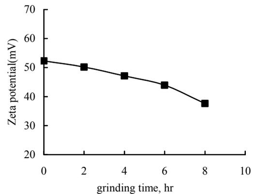
Figure 4. Effect of grinding time on Zeta potential
