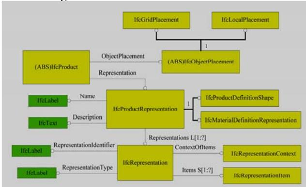
Figure 3 building component and geometric model integration.
