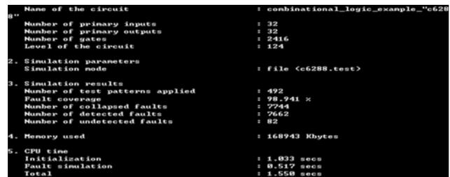
Figure 5. Results of Test Sequences Generated are Applied to ISCAS'85 Circuit
