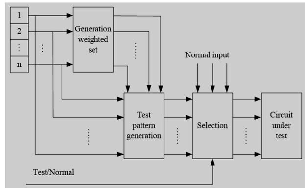
Figure 3. Structure Diagram of Test Pattern Generation
