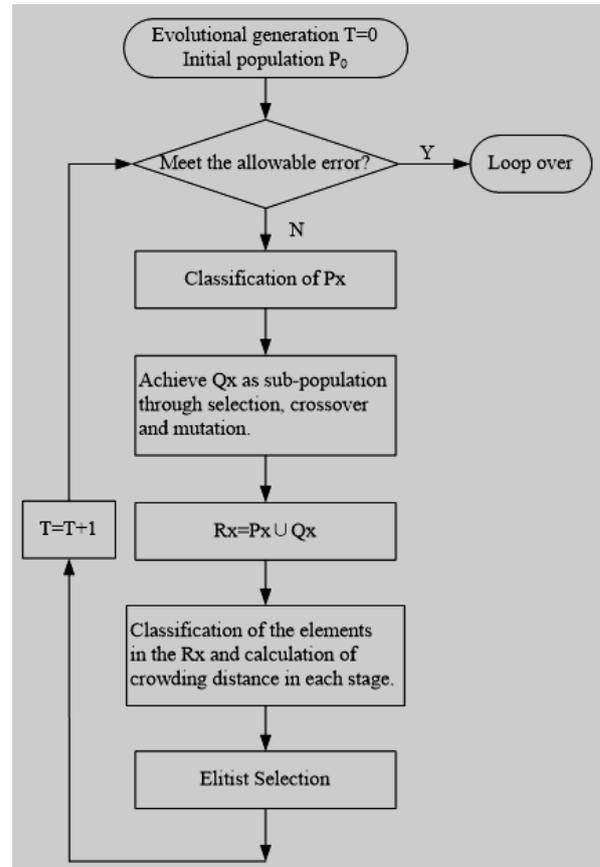
Figure 2. Multi-objective Genetic Algorithms Flowchart
