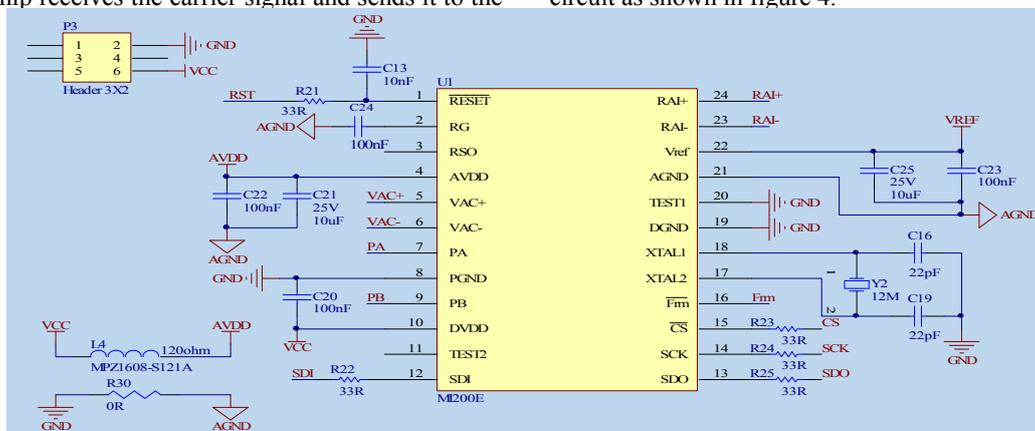
Figure 4. Chip circuit
