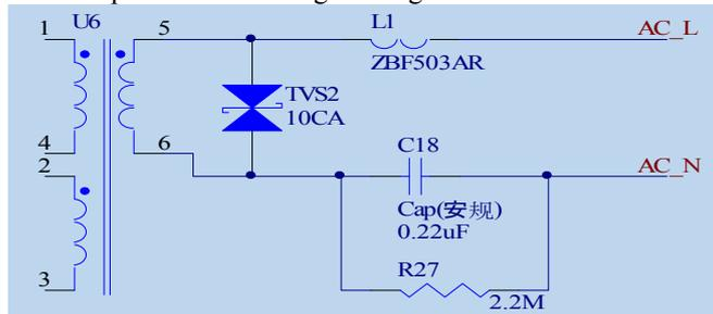
Figure 5. coupling circuit
