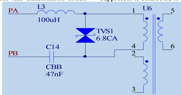
Figure 6. transmission filter circuit
