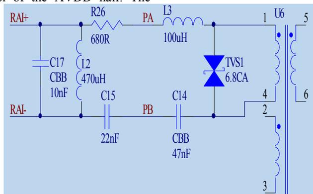
Figure 7. Receiving filter circuit
