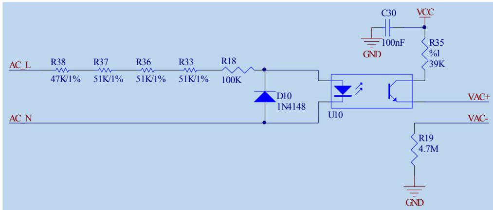
Figure 8. Zero crossing circuit
