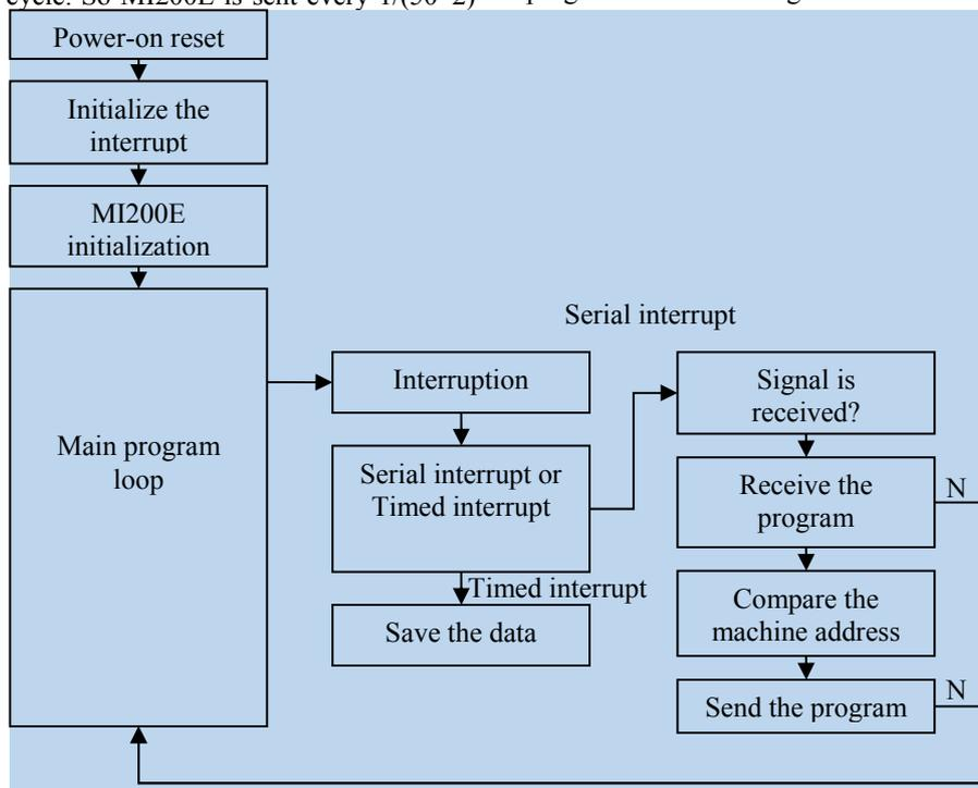
Figure 9. The main program block diagram
