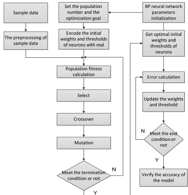
Fig 1. The procedure of BP neural network optimized by genetic algorithm
