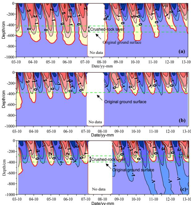
Figure 7. Freeze-thaw processes at the left shoulder boreholes of different structures. (a) CRBE; (b) CRSE; (c) UCRE.
