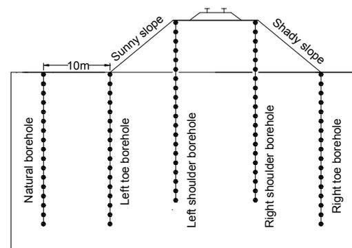
Figure 2. Location of temperature observation boreholes
