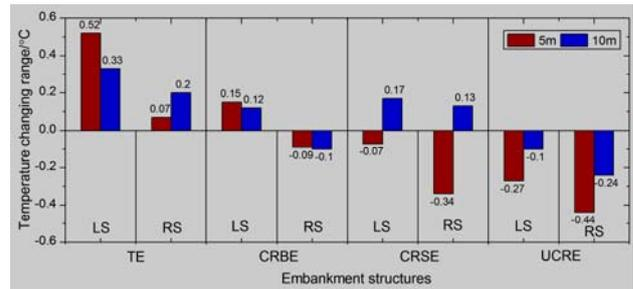
Figure 6. Variation range of permafrost temperatures at 5 m and 10 m under the two shoulders with different structures. (LS-left shoulder; RS-right shoulder).
