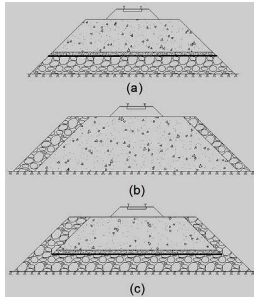
Figure 1. Structural diagrams of three types of crushed rock embankments. (a) CRBE; (b) CRSE; (c) UCRE;
