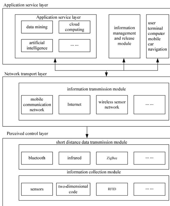
Figure 3. The underground logistics intelligent monitoring system based on the framework of internet of things.
