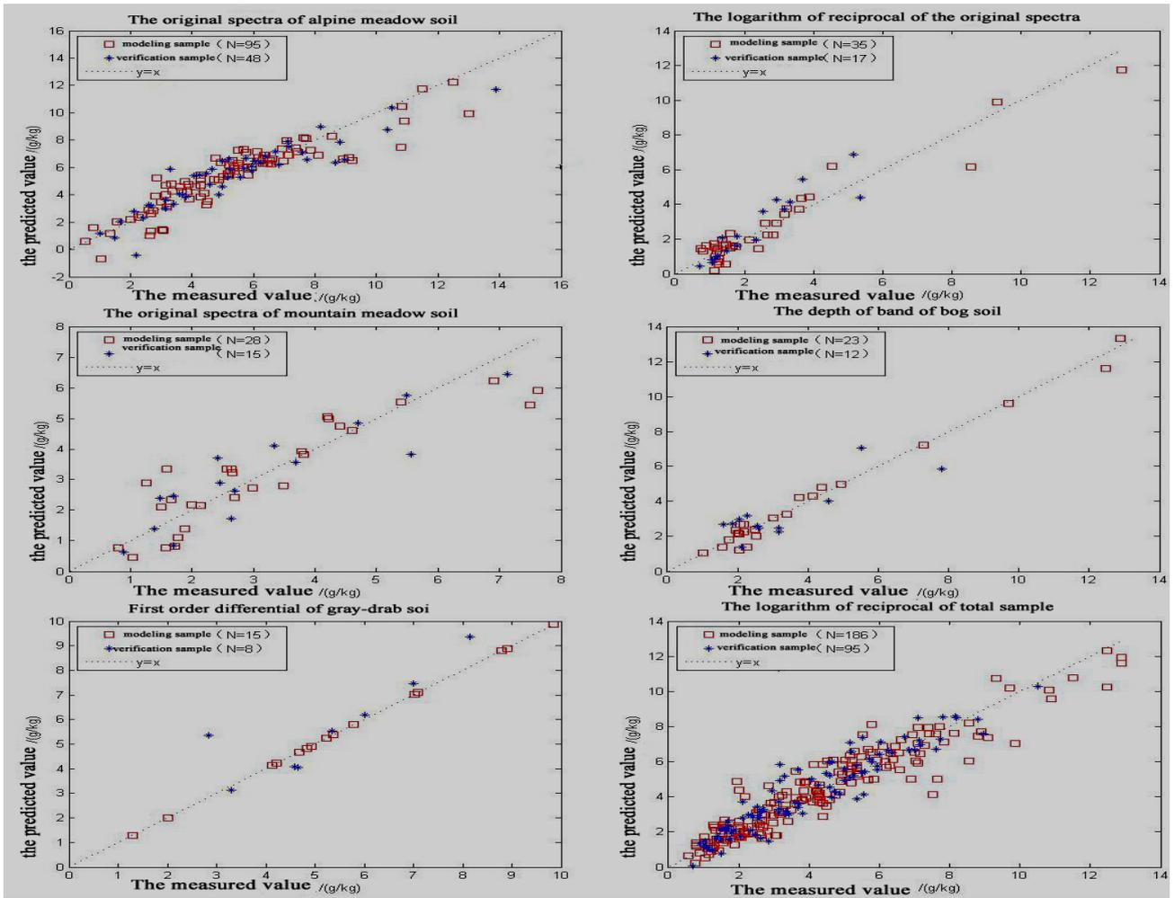
Fig.3 The Results of Full Band Model and Verification Accuracy of Total-Nitrogen of MSLR
