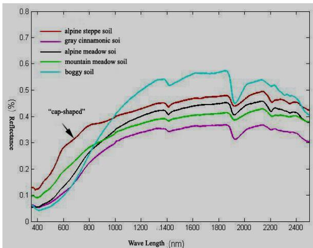
Fig.2 The Original Spectral Reflectance Curve of Various Soil Types
