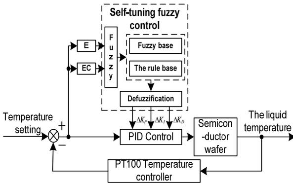
Fig.6 Self-tuning Fuzzy PID Control System Diagram
