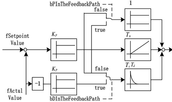
Fig.5 BECKHOFF Temperature Self-tuning PID Control Process
