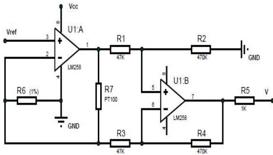
Fig.4 The Sampling Circuit of PT100
