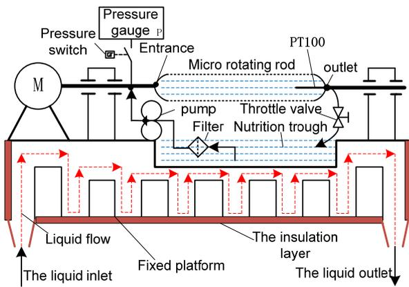
Fig.2 Two-Dimensional Design Diagram of Temperature Field
