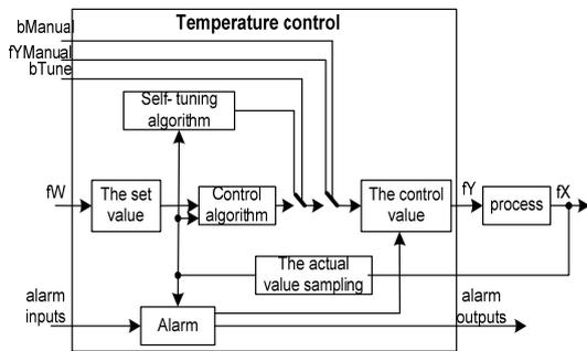
Fig. (8). The Diagram of BECKHOFF Open Temperature Control System
