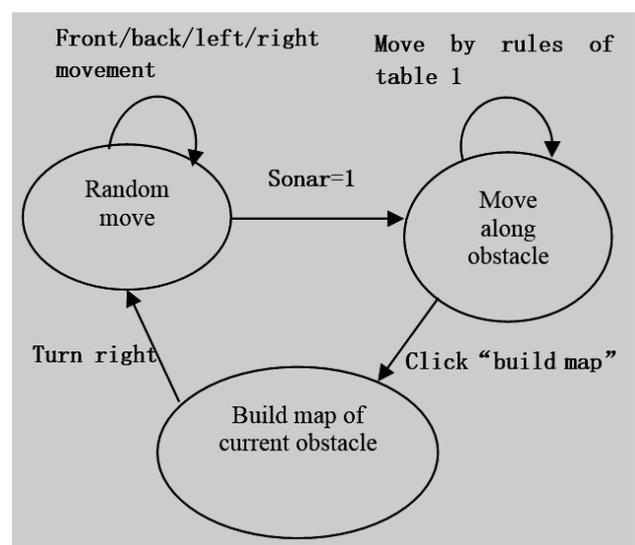
Fig.2 State Transition Diagram of Robot Movement
