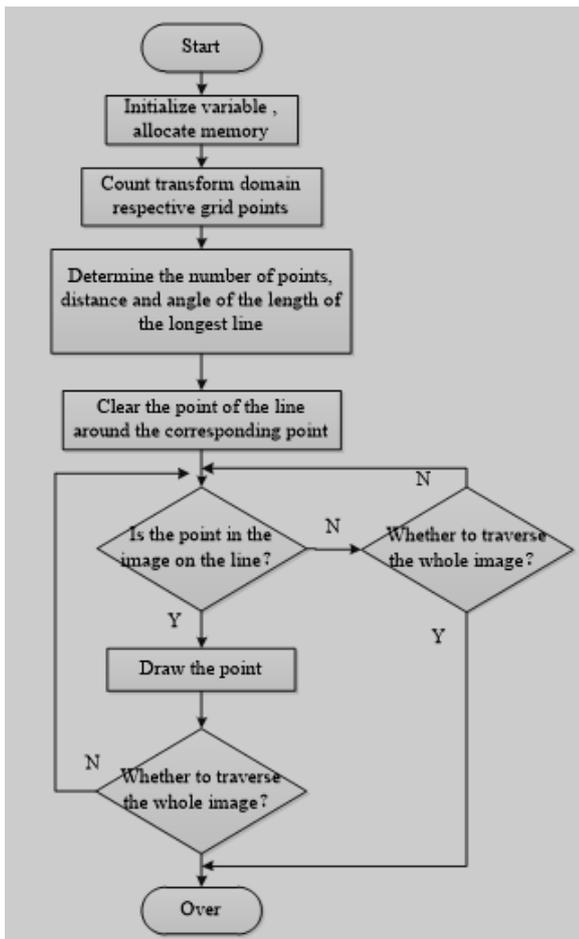
Fig.(2). The process of improved Hough transforms
