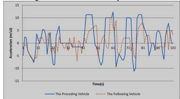
Fig.6 Acceleration Trend of the Two Vehicles
