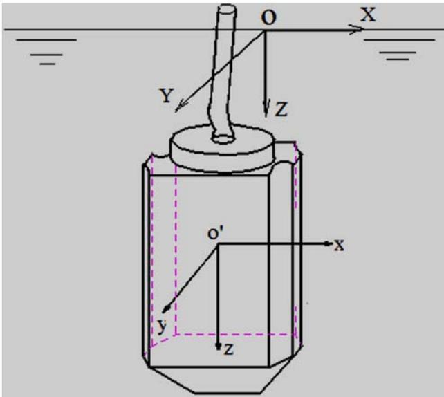
Figure 5. Coordinate system diagram of underwater robot.
