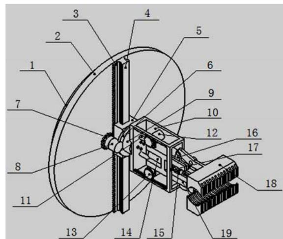
1. Disc-Shaped Rotating Motor 2. Rotating Disk 3. Lateral Moving Rack
