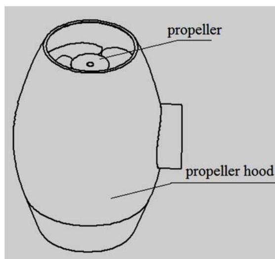
Figure 4. Propeller mechanism.
