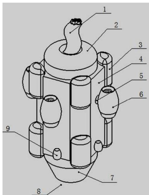
1. cable 2. cover 3. gasbag 4. shell 5. rotated motor 6. propeller mechanism 7. port 8. internal assembly 9. CCD outside the machine
