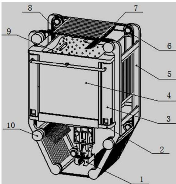
1. Gripper Moving Mechanism 2. Chassis 3. Adjusting Cylinder
