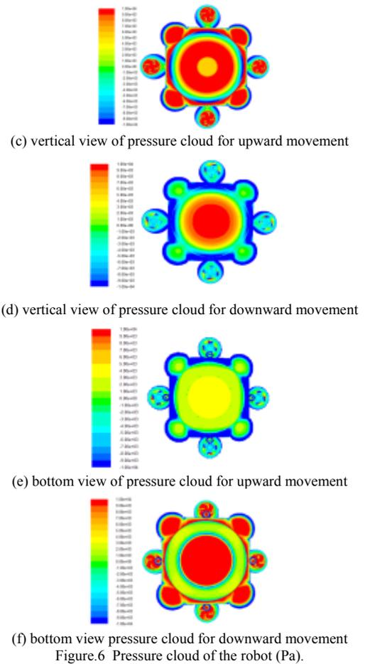
Figure.6 Pressure cloud of the robot (Pa).
