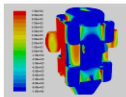
(a) Overall pressure cloud of the robot moving left
