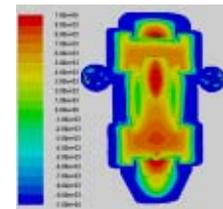
(c) Pressure cloud of the robot in outlet direction.
