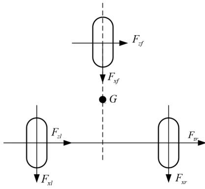
Fig.2 Friction Forces Suffered by Landing Gears
