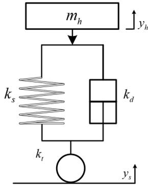
Fig.1 Refined Support Force Model
