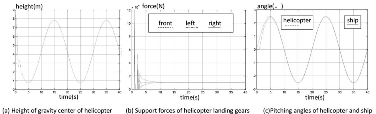
Fig.4 Simulation results in case 2
